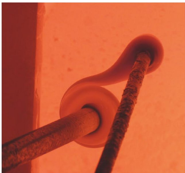
1. The core of the bracelet a bead is created by winding glass around a ferret.
