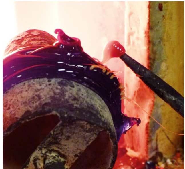
8. The wavy lines can be drawn with a cord of yellow glass.
