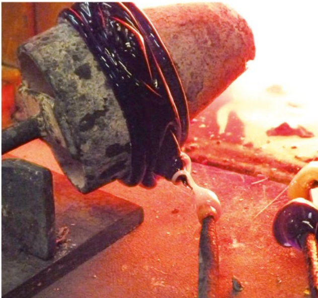
7. Yellow glass line is coiled around the protrusion. By warming up the bead protrusion shrinks.
