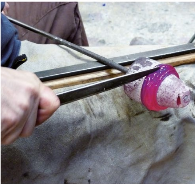
4. The ring is again incised on the sides and on the central ribs to create the losenge decoration.
