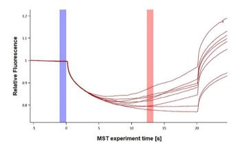
**Figure 3.** Thermographs of PD-1-eGFP in PBS-T buffer binding to PD-L1 at 37 °C. After 10 s of IR laser heating (MST power: 20%), a very large convection phenomenon was observed. The cold region is set to 0 s (blue) and the hot region to 12 s (red). The disturbance due to this event prevents the proper determination of a dissociation constant.
