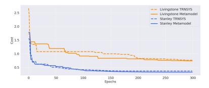
Figure 2: Calibration cost evolution for the metamodel and TRNSYS ( $\Delta_{\tt calib}$ , see 2), on Livingstone and Stanley. Both models were calibrated for 300 epochs, which is enough to reach convergence for Stanley, but not Livingstone.
