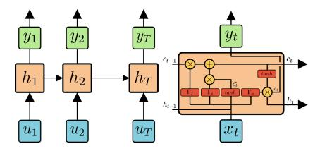
Figure 1: Our metamodel architecture (left), and a detailed LSTM cell (right). The LSTM cell improves on the classic RNN by introducing a cell state  $c_t$  supposed to carry long term memory, without additional alterations, throughout the sequence. The three input gate  $\Gamma_i$ , forward gate  $\Gamma_f$  and output gate  $\Gamma_o$  determine whether information in both hidden state  $h_k$  and cell state  $c_k$  should be carried away or discarded.
