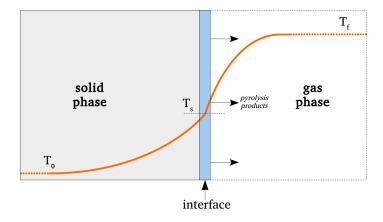
Figure 1: 1D model of a solid propellant burning
