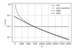
Figure 7: Regression speed as a function of activation temperature, CFD results compared to semi-analytical and analytical results
