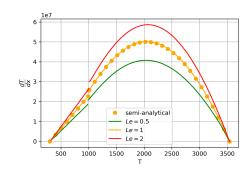
Figure 10: Phase portraits, CFD results (full lines) compared to semi-analytical results (dots)
