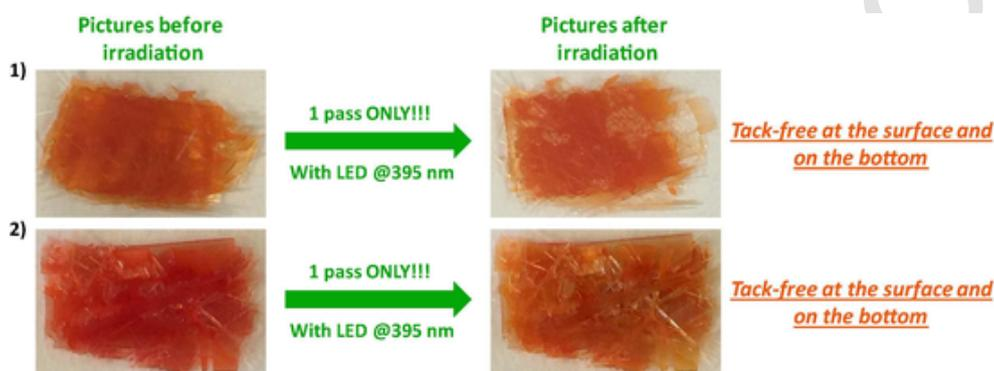
Fig. 22. Photocomposites obtained with a LED conveyor at 395 nm (belt speed : 2 m/min), using a glass fibers/(meth)acrylate resin (50%/50%) : (1) 0.05% **PP41** + 1% Iod + 1% NPG in BisGMA/TEGDMA; (2) 0.05% **PP40** + 1% Iod + 1% NPG in TMPTA. Adapted from ref. [97] with permission from The Royal Society of Chemistry.
