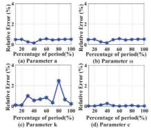
Fig. 6. The difference of JA parameters achieved by percentage of period compared to initial JA parameters
