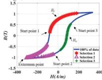
Fig. 8. Uncomplete hysteresis loop with different start point for identification
