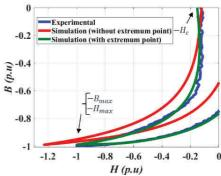
Fig. 12. Comparison of experimental and simulated hysteresis cycles
