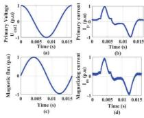
Fig. 10. (a) Measured primary voltage of transformer  $(U_{cat_2})$ , (b) Measured primary current of transformer  $(I_p)$ , (c) Calculated magnetic flux of transformer  $(\emptyset_m)$  and (d) Calculated magnetizing current of transformer  $(I_m)$
