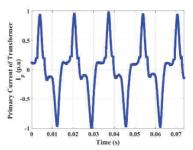
Fig. 9. (a) Measured primary current of transformer  $(I_p(A))$
