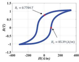
Fig. 4. Hysteresis loop of transformer with the JA parameters in table I.
