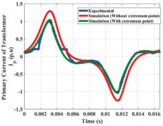
Fig. 13. Comparison of simulation result and experimental measurement of primary current
