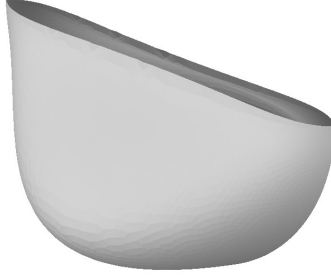
FIGURE 6. Optimal hull built on a half disc for Fr = 1.75 (3D view of Figure 5-top)
