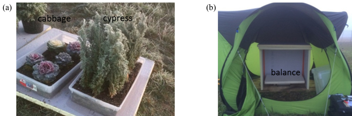
Fig. 2. Experimental set-up of the weighing method: (a) plastic containers each containing one of the three plant species; (b) balance (without plants) under a shelter to prevent weighing disturbances from wind fluctuations.
