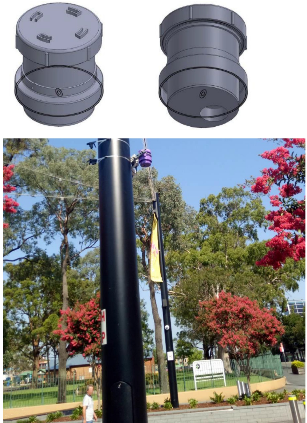
Fig 2. Housing of the air quality device (top images) and installed (purple coloured) on pole in Liverpool Mall (images: top, S. Selby; bottom, H. Forehead).
