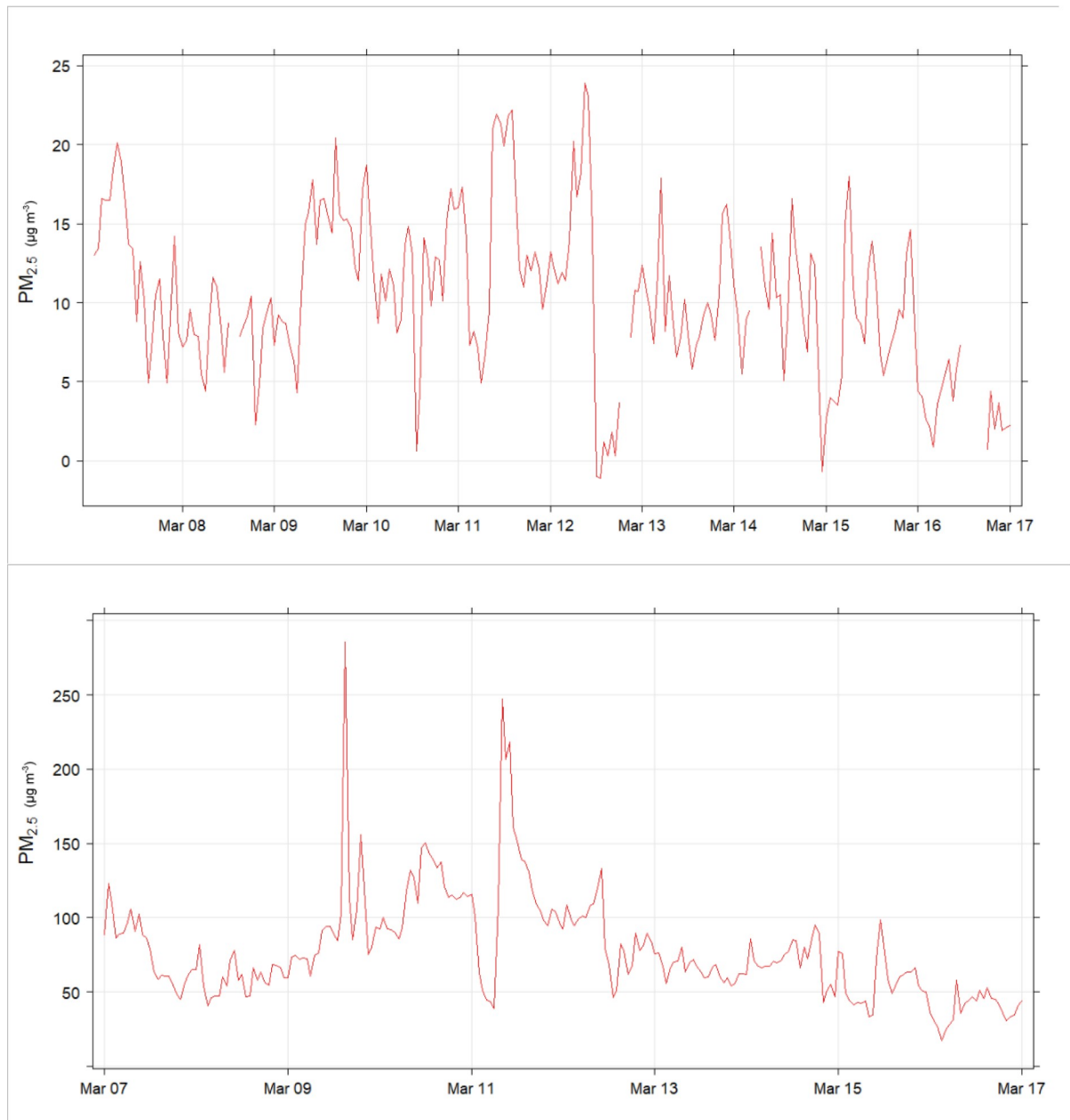
Fig 7. Time series plots showing differences in hourly PM_{2.5} readings ( \mu g m^{-3} , note different scales) between an air quality monitoring station and at street-level, over 9 days in March 2019. Averaging period 1 hr. There was no pollution from bushfires in the time shown. (top) Department of Planning, Industry and Environment (DPIE) air quality monitoring station in Pearce Park, Liverpool. (bottom) AQ9 at the corner of Bigge St & Scott St, a "T" intersection near the train station, 1.9 km ENE of Pearce Park.
