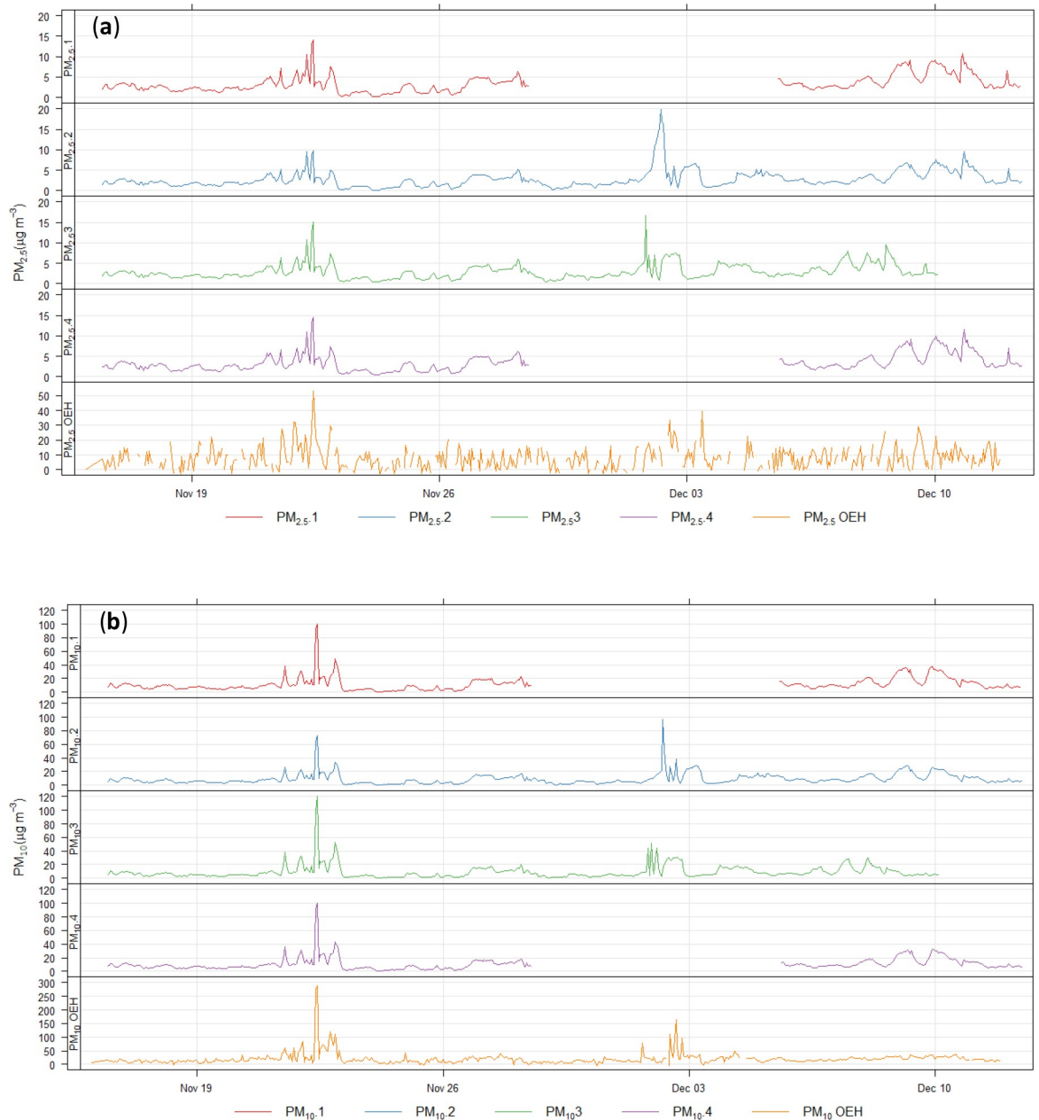
Fig 5. Hourly averaged PM measurements ( \mu\text{g m}^{-3} , note different scales) from 4 devices co-located with Department of Planning, Industry and Environment (DPIE) reference instrument in December 2018. (a) \text{PM}_{2.5} 1–4, \text{PM}_{2.5} DPIE and (b) \text{PM}_{10} 1–4, \text{PM}_{10} DPIE; at DPIE air quality monitoring station in Campbelltown, western Sydney. Missing data in plots 1 & 4 due to power failure, time lag in 3 from early December due to a failing battery in the device's clock.
