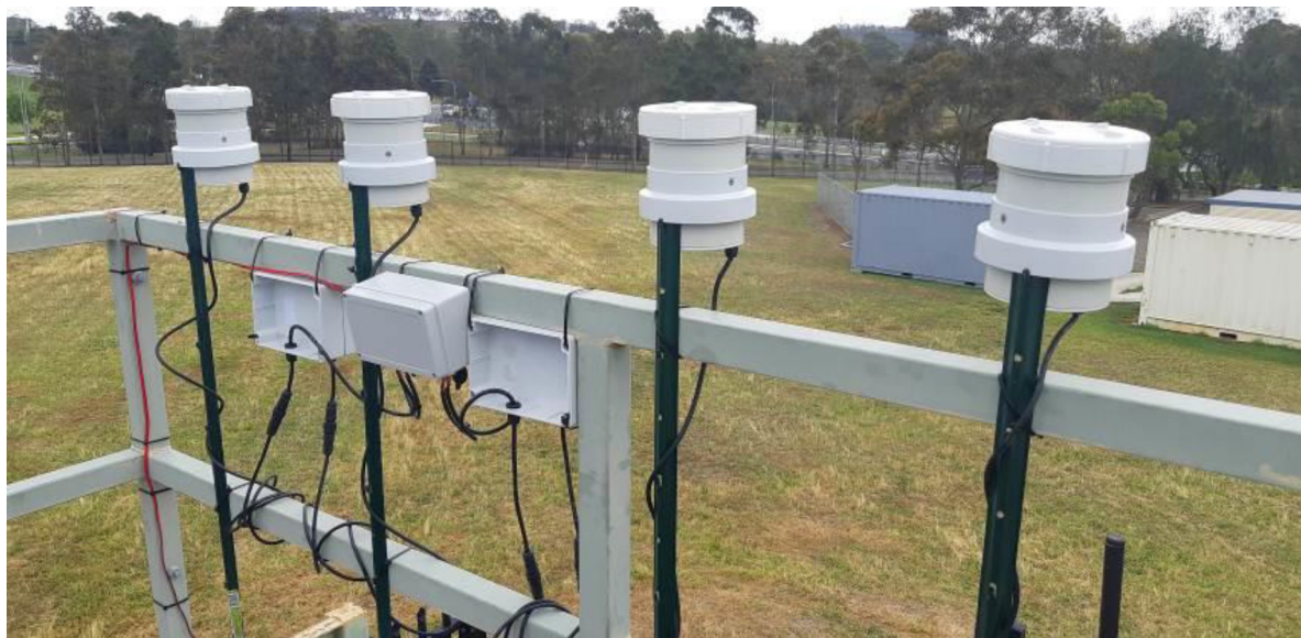
Fig 3. PM measuring devices under test at Department of Planning, Industry and Environment (DPIE) Campbelltown West air quality monitoring station (image: O. Price).
