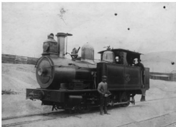
Figura 5. Locomotora Kitson-Meyer de Taltal. AMACR
