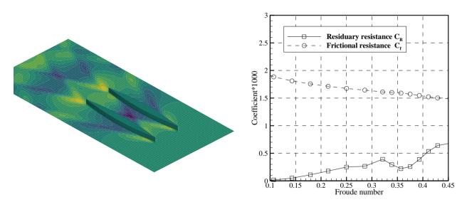
Figure 12Picture of the hull shape considered in this study and related hydrodynamic coefficientsFig. 12 shows the shape and resistance coefficients of the proposed energy ship hull, whose displacement is 660 t. The shapeof the floaters is based on the Wigley hull, which is defined by:
