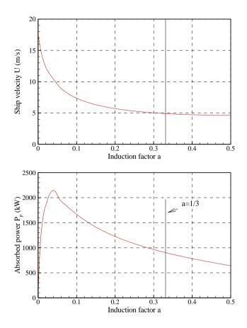
Figure 5 Ship velocity (top) and absorbed power (bottom) as function of the induction factor. The true wind speed is 10 m/s and 215 the true wind angle is 90°. The wind propulsion subsystems are Flettner rotors. The spin ratio is 3. Constraints on maximum rotational velocity, maximal thrust and cut-out speed are not taken into account in this example.
