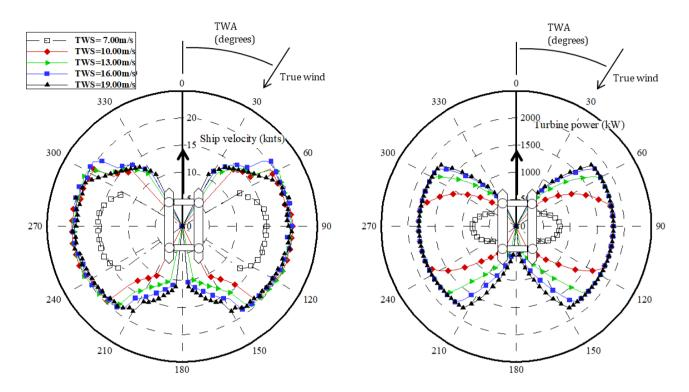
Figure 13 Velocity (left) and generated power (right) polar plots of the proposed energy ship design for true wind speeds of 7, 10, 13, 16 and 19 m/s. TWA stands for true wind angle.
