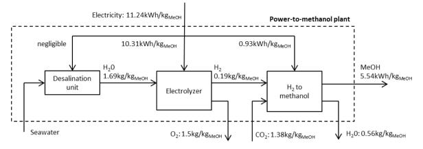
Figure 7 Assembled model for the power-to-methanol plant
