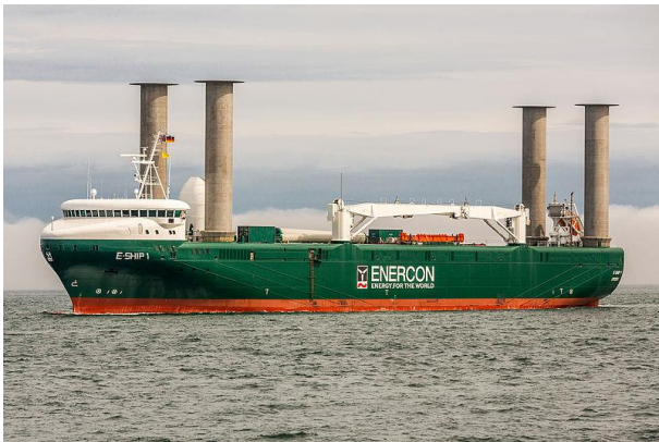
Figure 9 On the left, the “E-Ship 1” in 2015. It is fitted with four 27 m tall Flettner rotors. Picture by Alan Jamieson. On the right, diagram showing the Magnus effect by which lift is produced by a rotating cylinder.
