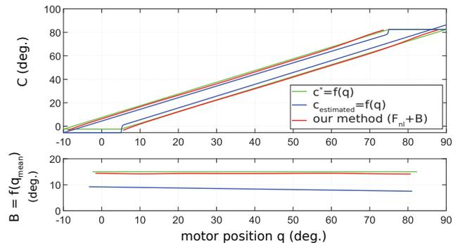
Fig. 7. Reconstructed hysteresis (top) and backlash width function (bottom) as a function of  $q$ . The robot is simulated with a constant  $15^\circ$  backlash on the bending joint, and a  $\pm 1.5^\circ$  error on the hand-eye calibration. Green: ground truth, Blue: Direct single-step estimation of the hysteresis using pose estimation, Red: using the proposed approach.
