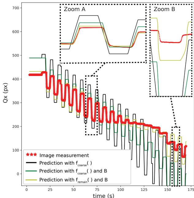
Fig. 10. Pseudo-periodic trajectory used for testing prediction capability of different models:  $f_{coarse}$  (black),  $f_{coarse} + B$  (green) and  $f_{remain} + B$  (yellow). Zooms A and B show that when backlash is modeled the appearance of motion is well synchronized with the measurement.
