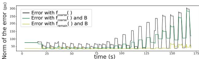
Fig. 11. Reprojection errors between the measured position of the effector in the endoscopic image and the prediction of effector position provided by  $f_{coarse}$  (black),  $f_{coarse} + B$  (green) and  $f_{remain} + B$  (yellow).
