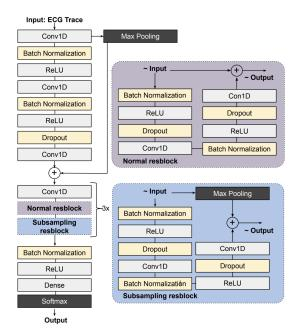
Fig. 5: ECG Convolutional Neural Architecture.
