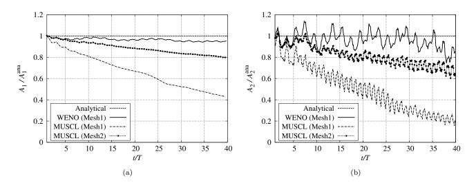
Figure 15: Moving-window fast Fourier transform of the free-surface elevation  $\eta_m(t) = \eta(L/2, t)$ : (a) 1<sup>st</sup>-harmonic amplitude  $A_1/A_1^{\text{ana}}$  with  $A_1^{\text{ana}} \simeq 2.8166 \times 10^{-2}$  m; (b) 2<sup>nd</sup>-harmonic amplitude  $A_2/A_2^{\text{ana}}$  with  $A_2^{\text{ana}} \simeq 3.3283 \times 10^{-3}$  m.
