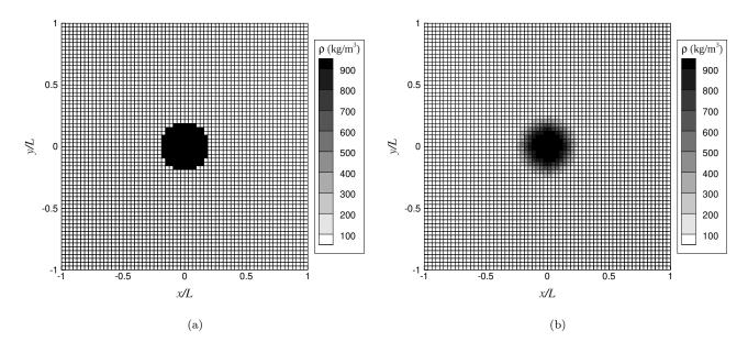
Figure 6: Density fields of the mixture in the 2D interface advection test-case: (a) t = 0 s; (b) t = 1 s.
