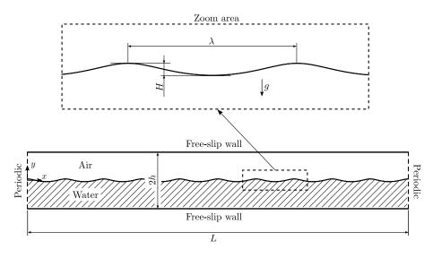
Figure 12: Configuration of the wave propagation test-case.
