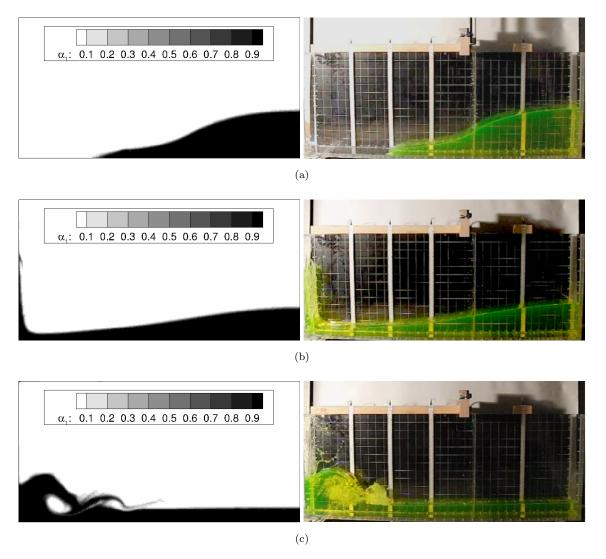
Figure 17: Comparison of flow patterns between the numerical results (left) obtained with the proposed WENO scheme and the experimental measurements (right) carried out by Lobovsky et al. [23] (reprinted with permission from Elsevier) at three dimensionless instants  $t^* = t\sqrt{g/H}$ : (a)  $t^* \simeq 1.58$ ; (b)  $t^* \simeq 3.27$ ; (c)  $t^* \simeq 6.67$ .
