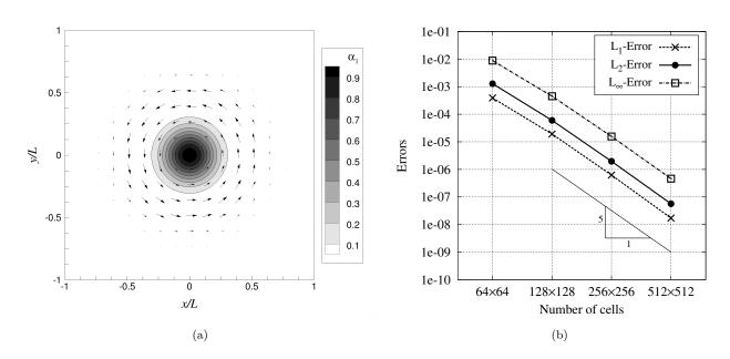
Figure 8: 2D multiphase vortex advection test-case: (a) initial configuration in the moving frame; (b) convergence order.
