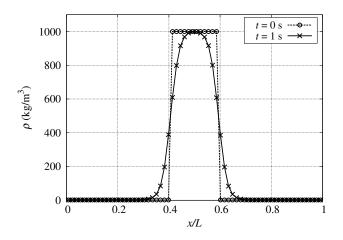
Figure 3: 1D interface advection test-case: density of the mixture at t = 0 s and t = 1 s.
