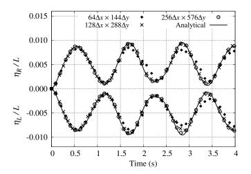
Figure 10: Time history of the interface elevations  $\eta_L = \eta(0, t)$  and  $\eta_R = \eta(L, t)$  on the left and right walls in the linear sloshing test-case with three mesh resolutions:  $64\Delta x \times 144\Delta y$ ,  $128\Delta x \times 288\Delta y$  and  $256\Delta x \times 576\Delta y$ .
