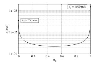
Figure 1: Speed of sound in an air-water mixture with  $\rho_1 = 1000 \text{ kg/m}^3$ ,  $\rho_2 = 1 \text{ kg/m}^3$ ,  $c_1 = 1500 \text{ m/s}$  and  $c_2 = 350 \text{ m/s}$ .
