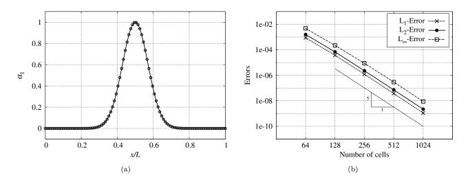
Figure 5: Convergence study in the 1D advection test-case: (a) initial volume fraction field; (b) convergence order.
