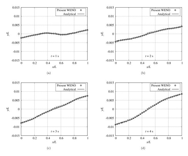
Figure 11: Shape of the air-water interface in the linear sloshing test-case using the mesh resolution  $256\Delta x \times 576\Delta y$  at four instants: (a) t = 1 s; (b) t = 2 s; (c) t = 3 s; (d) t = 4 s.
