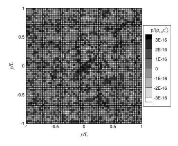
Figure 7: Pressure field at the final instant (t = 1 s) in the 2D interface advection test-case.
