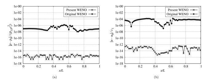
Figure 4: 1D interface advection test-case carried out with the present and original WENO schemes at t = 1 s: (a) pressure field; (b) velocity field.
