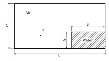
Figure 16: Initial configuration of the dam-break flow test-case.
