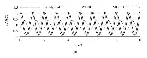
Figure 13: Shape of the free-surface in the wave propagation test-case using the proposed WENO scheme and the MUSCL scheme with the same mesh of resolution  $1024\Delta x \times 512\Delta y$  at four instants: (a) t = 10T; (b) t = 20T; (c) t = 30T; (d) t = 40T.
