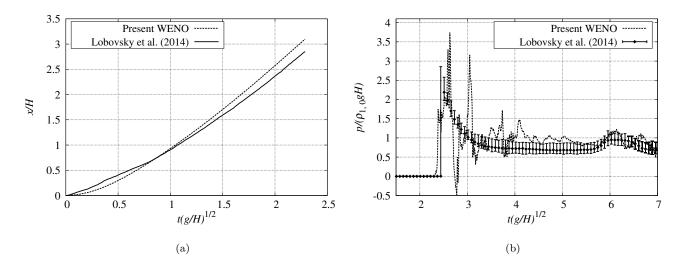
Figure 18: Water front position and pressure signal in the dam-break flow test-case: (a) time history of the water front position; (b) pressure signal at the left lower corner of the tank.
