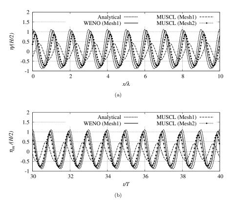
Figure 14: Numerical result obtained with the MUSCL scheme using the refined mesh (Mesh2:  $2048\Delta x \times 1024\Delta y$ ): (a) shape of the free-surface at t = 40T; (b) time evolution of the free-surface elevation  $\eta_m(t) = \eta(L/2, t)$  during the last 10 wave periods.
