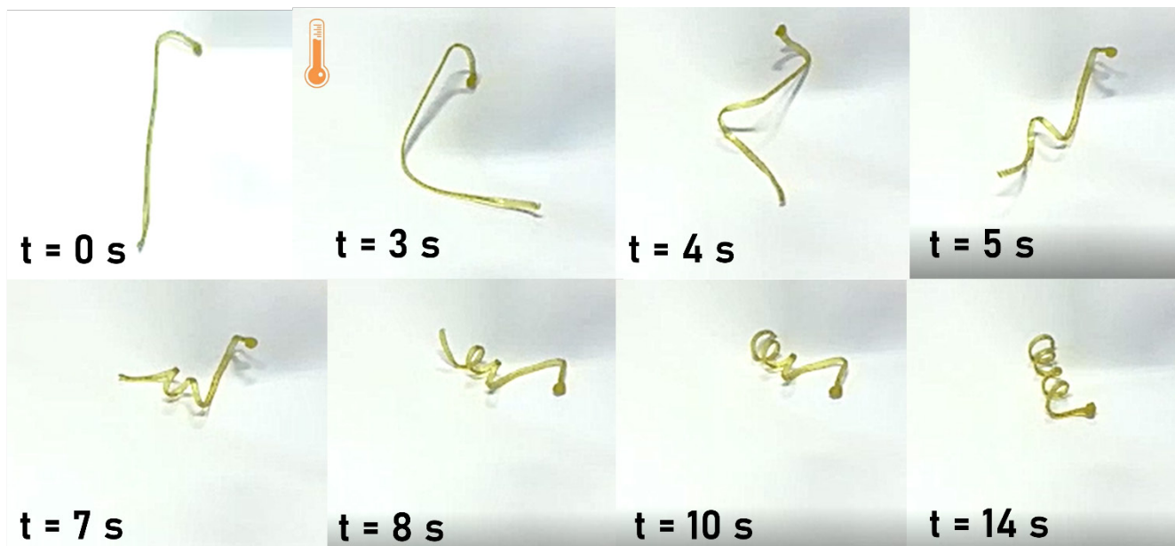
Figure 4. Shape memory behavior demonstration on PHU 30 . A strand of PHU 30 cured in a helical shape is deformed into a straight shape and cooled at -20 °C. Upon heating at 80 °C (heat gun) the initial shape is recovered in 14 seconds.
