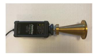
Figure 7. Open-ended coaxial probe.
