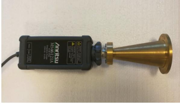
**Figure 7.** Open-ended coaxial probe.
