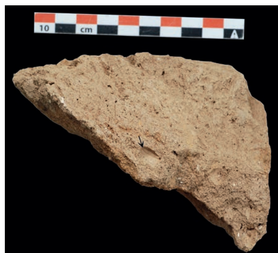
Fig. 5. Mud-brick 35315_Bot1. Detail of the plant temper. Imprints of beetle (arrow).
