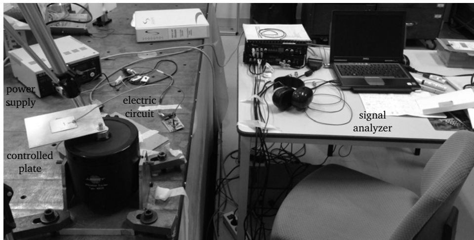
35 Figure 5: Layout of the measurement system for a single patch. The controlled aluminum 36 plate measures 70 \times 70 \times 3 \text{ mm}^3
