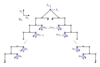
Fig. 1: Kinematic structure of the DiMiBot, with 2*N* bistable modules.
