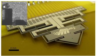
Fig. 2: Digital microrobot containing 4 bistable modules (N = 2), and a zoom view of the end-effector while manipulating a 150  $\mu m$  diameter glass ball.
