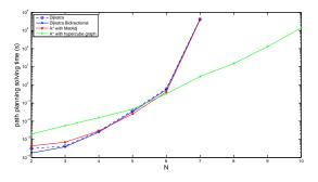
Fig. 12: Comparison in computation time for the different algorithms in the cases for robots up to 20 bistable modules (N = 10).
