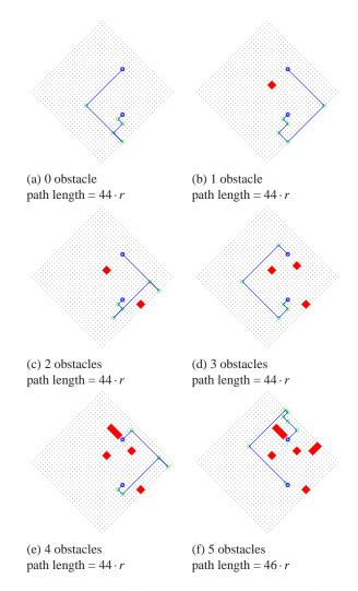
Fig. 9: Shortest path found with the Dijkstra's algorithm in the case of a DiMiBot with 10 bistable modules (N = 5) and with the presence of 0 to 5 obstacles.
