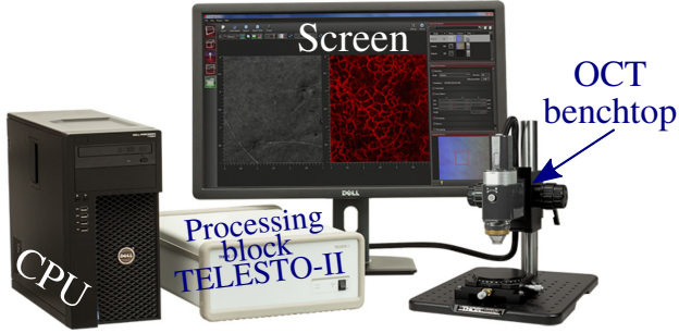
Fig. 7. Global view of the OCT acquisition setup.
