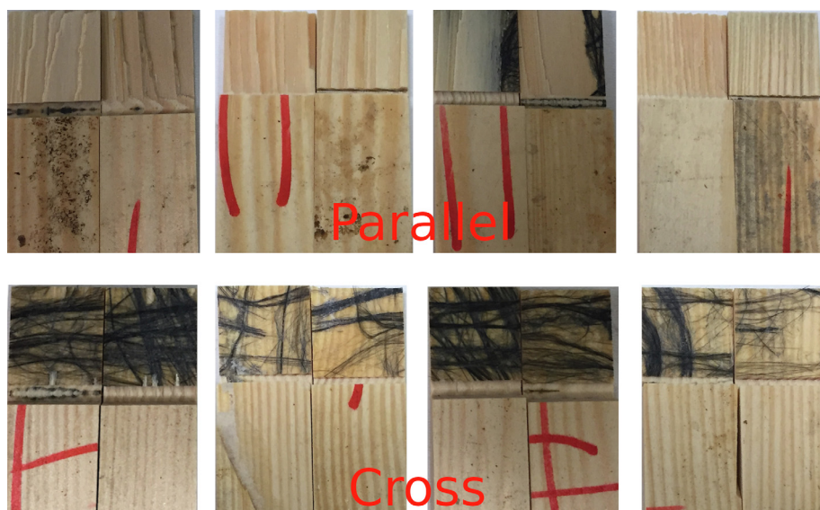
Fig. 6. Bond section of shear strength samples after testing.
