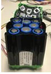
Fig.7. Module of 8 Li-ion LFP cells developed by TYVA ENERGY.
