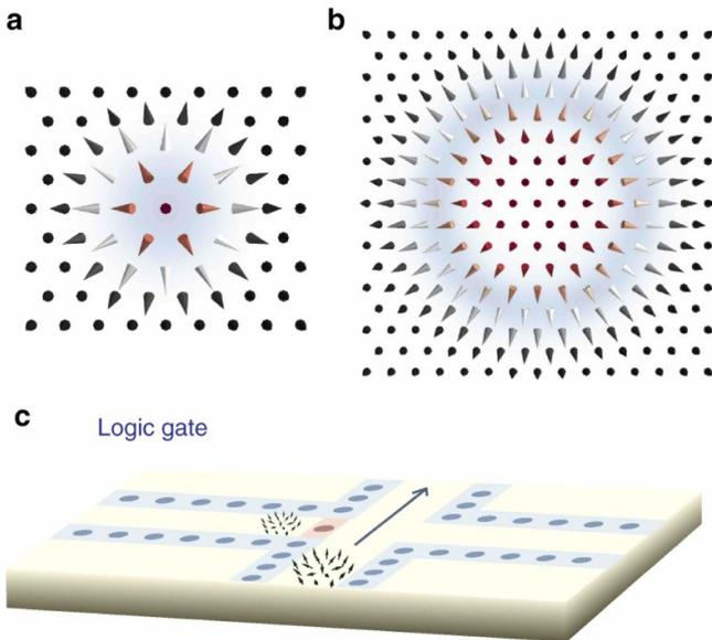
**Figure 11.** Spintronic devices with defects guiding the motion of a skyrmion. (a), (b) Non-collinear regions (blue area) defining pinning or repulsion depending on the chemical nature of the impurities. A pinning impurity can lock a skyrmion within the blue region while a repulsive impurity can pin a large skyrmion on the core region, which is a local minimum energy. (c) Pinning (red) usually hinders skyrmion mobility and can be used to decelerate them. Reproduced from [89]. CC BY 4.0.
