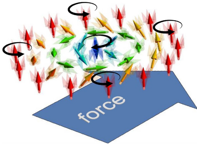
Figure 10. When a force is applied to a skyrmion, internal degrees of freedom are excited. These internal excitations lead to retardation effects which can be described as an effective mass of the skyrmion. Different forces lead to different types of deformations and therefore to different values of the effective mass. Reproduced from [88].
