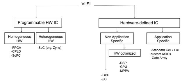
Fig. 1. Taxonomy on VLSI Integrated Circuits
