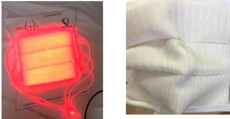
*Figure 13: PAGETEX® device connected with 635 nm LASER source – flat device (Left), folded device (Right)*
