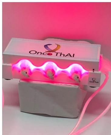
*Figure 10: VIVO-LEF can illuminate 3 mice simultaneously with homogeneous light*
