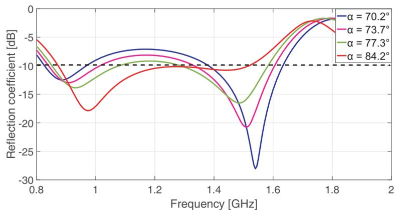
**Figure 7.**  $S_{11}$  of the proposed antenna as the function of frequency with different values of ( $\alpha$ ).
