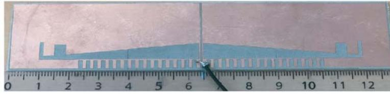
**Figure 8.** Photograph of manufactured antenna with Taconic RF-35.
