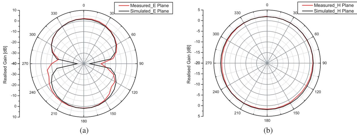
**Figure 11.** Simulated and measured (a) *E*-plane, (b) *H*-plane of the proposed antenna in free space at 868 MHz.
