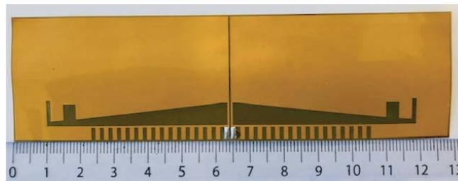
**Figure 15.** Photograph of manufactured antenna with Kapton.
