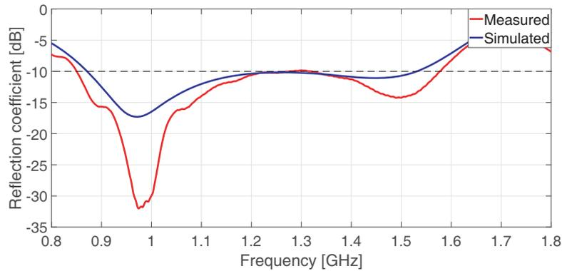
**Figure 9.** Simulated and measured  $S_{11}$  of the proposed antenna in free space.
