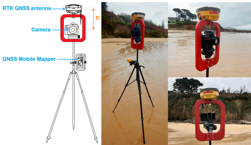
Figure 2. Measurement system developed for the Real Time Kinematic (RTK) Global Navigation Satellite System (GNSS)-assisted terrestrial Structure-from-Motion (SfM) photogrammetry method (equipped with the Nikon D800 Reflex camera or with the Huawei Y5 Smartphone).
