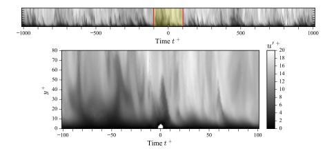
Figure 5: Time trace of streamwise velocity u' at  $U_{\infty}=5\,\mathrm{m/s}$  ( $Re_{\theta}=4767,~X=6.8\,\mathrm{m}$ ) covering 0.75 s (5000 samples, top) and 0.075 s (5000 samples, bottom). The white region at time  $t^+=0$  indicates a single reverse flow event. In both sub-plots the vertical axis represents wall distance  $0< y<80^+~(\approx 6\,\mathrm{mm})$ .
