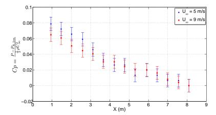
Figure 1: Streamwise pressure coefficient distribution on the wind tunnel top wall for the two studied free stream velocities with respect to pressure measurement at  $X=8.1\,\mathrm{m}$ .
