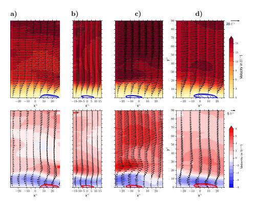
Figure 10: Various instances of near wall reverse flow obtained at measurement position  $x=3.2\,\mathrm{m}$  at  $Re_\theta=2537$  (a,b) and  $Re_\theta=4000$  (c,d). Bottom row is plotted in fluctuating velocity (mean local streamwise velocity subtracted).
