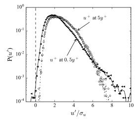
Figure 4: Probability density functions of the fluctuating streamwise velocity  $u^+$  at wall distances of  $0.5\,y^+$  and  $5\,y^+$  for  $Re_\theta=2537~(X=3.2\,\mathrm{m})$ .
