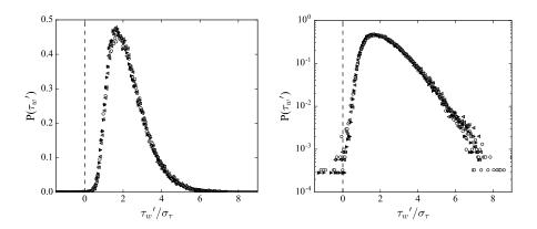
Figure 3: Probability density functions of wall shear stress  $\tau_w$  for three separate image sequences obtained for  $Re_\theta=4000~(X=3.2\,\mathrm{m})$  in linear (left) and logarithmic scaling (right).
