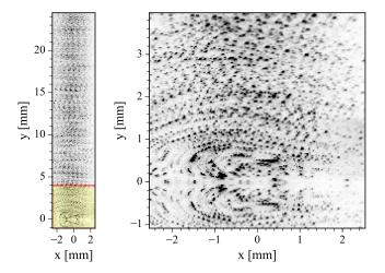
Figure 6: Multi-exposed particle images showing a near wall flow reversal event in a ZPG TBL at  $Re_\theta=4767~(X=6.8\,\mathrm{m},\,U_\infty=5\,\mathrm{m/s})$ . Full image view at left with detail on right. The tunnel glass wall is located at Y=0 with reflections of particle images visible at Y<0.
