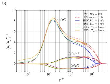
Figure 2: Profiles scaled with inner variables of the mean streamwise velocity (a) and Reynolds stresses (b) for two different free stream velocities obtained  $X=6.8\,\mathrm{m}$  downstream of the tripping device.
