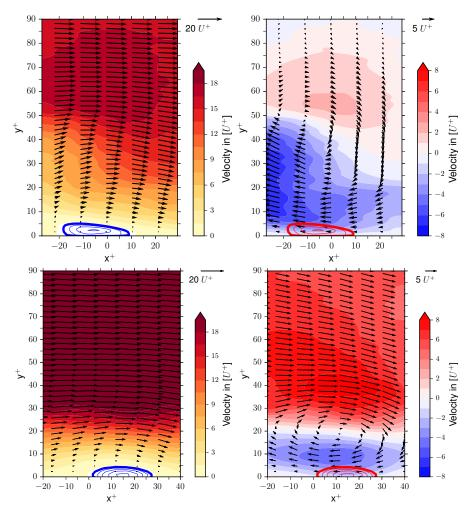
Figure 8: Single reverse flow events at  $Re_{\theta}=4767$  (top) and  $Re_{\theta}=7952$  (bottom) shown in viscous scaled units (left) and with mean local streamwise velocity subtracted (right). Contours near y=0 represent horizontal velocity  $U\leq 0$  at increments of  $0.2U^+$ .
