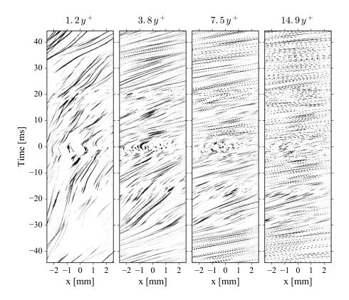
Figure 7: Particle streaks extracted at various wall-normal distances at  $U_{\infty}=5\,\mathrm{m/s}$  ( $Re_{\theta}=4767$ ) covering 0.1 s (667 samples; 274  $t^+$ ) on vertical axis. A single reverse flow event is located near t=0.
