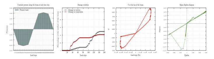
Figure 23: TC Model: tension-compression cycle. P,  $\chi$ , U et  $\sigma/\varepsilon$  (values of  $\sigma$  and  $\epsilon$  are taken at the central point).
