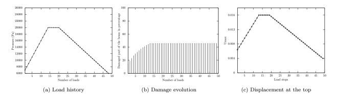
Figure 9: Load history, percentage of damaged beam and maximum bending
