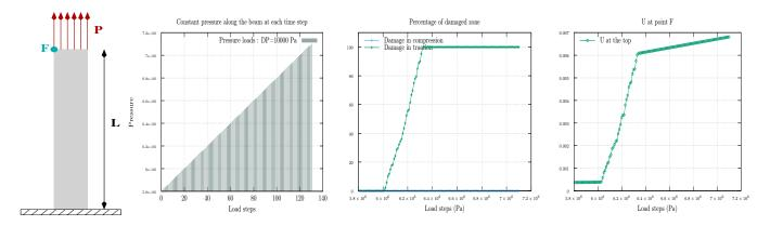
Figure 10: Tension-Compression model: configuration of the tension experiment (left), pressure load (center left), damage function in percentage (center right) and the displacement U at the F point (right).
