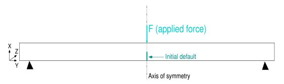
Figure 28: Configuration of the three-point flexural experiment
