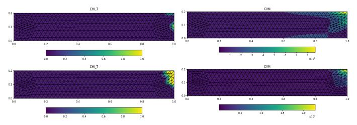
Figure 31:  $\chi$  in tension (left) and VMS (right) fields during the propagation of the damage
