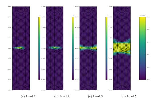
Figure 16:  $\chi_t$  evolution from the first damage state with an initial default
