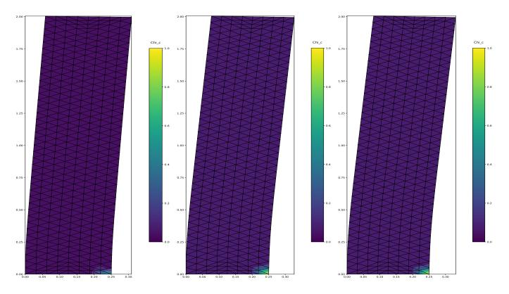
Figure 37: Damage area in compression:  $\chi_t$  field at loads 18, 20 and 21
