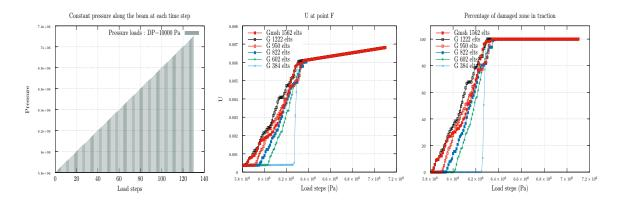
Figure 11: Comparison between different sizes of mesh with constant  $\Delta P = 10000 \,\mathrm{Pa}$ : scenario of charge (left), displacement (U) at the top point (center) and damage evolution in percentage (right).
