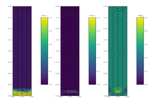
Figure 20: TC Model: tension-compression cycle.  $\chi_t$  (left),  $\chi_c$  (center) and VMS field (right) at load 32.
