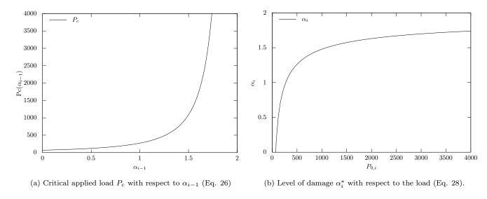
Figure 4: Evolution of the critical load, function of the previous state  $\alpha_{i-1}$  (left) and evolution of the damage state, function of the load  $P_{0,i}$  (right).
