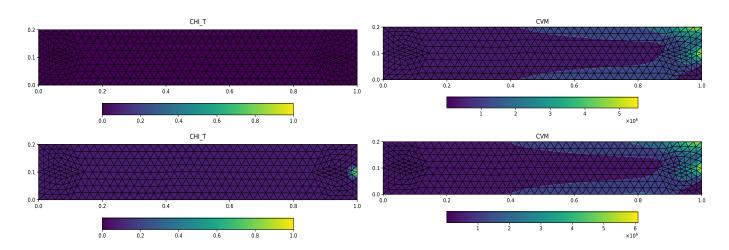
Figure 30:  $\chi$  in tension (left) and VMS (right) fields at the onset of the damage
