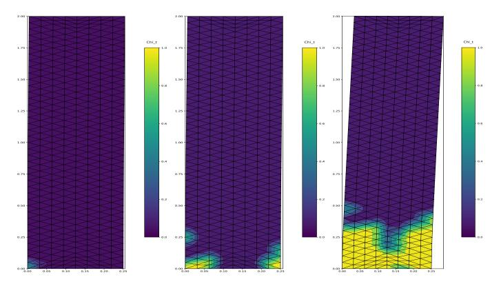
Figure 35: Damage area in tension:  $\chi_t$  field at loads 9, 11 and 14
