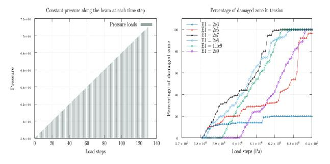
Figure 13: P,  $\chi_t$  for the tension experiment with different values of  $E_1$  parameters from  $2.10^9$  Pa to  $2.10^3$  Pa
