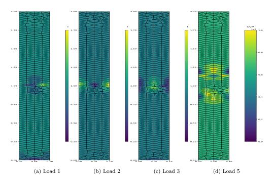
Figure 17: Corresponding VMS evolution during the tensile test with an initial default
