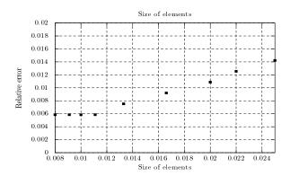
Figure 5: Relative error for the critical pressure  $P_{\min}$  with respect to the mesh size.
