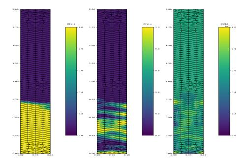
Figure 22: TC Model: tension-compression cycle.  $\chi_t$  (left),  $\chi_c$  (center) and VMS field (right) at load 99.
