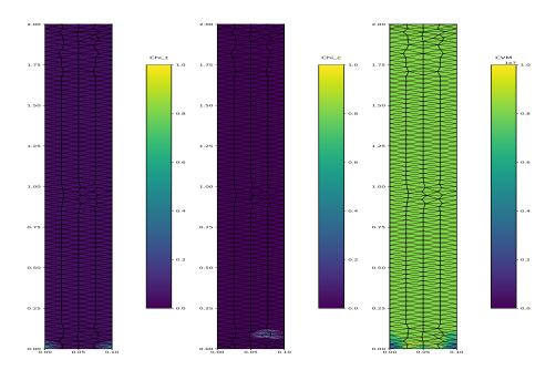
Figure 19: TC Model: tension-compression cycle.  $\chi_t$  at load 29 (left),  $\chi_c$  at load 31 (center) at the onset of the damage and corresponding VMS field (right, load 30).
