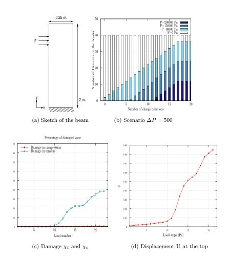
Figure 33: Load schemes and damage zone of the beam
