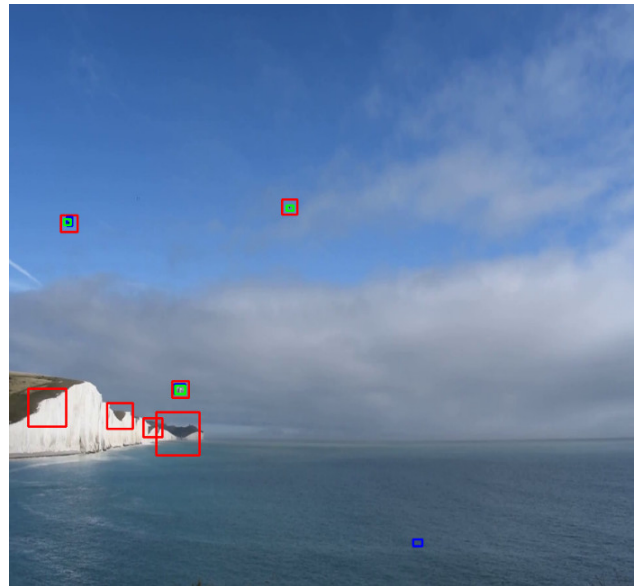
Figure 6. True Positive and False Alarm Rates for small aerial object detection with a lightweight YOLO based detector and conventional methods. There exists 1 drone (green box at the bottom) and two birds (green boxes at top) in the scene. Detections by lightweight YOLO, cascaded HAAR and background subtraction are depicted with green, red and blue boxes, respectively. Note that, cascaded detector produces a lot of false alarms, whereas waves on sea causes false alarms for background subtraction. Footage taken from experiments by [25]
