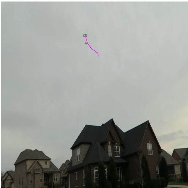
Figure 8. The aerial object detection and tracking with Kalman filtering. Based on the movements of the target, the system is activated, turret is rotated towards it and the object is classified as drone or not with a zoomed daylight and thermal camera.
