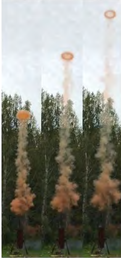
Figure 14: High speed camera diagnostics of vertical movement of the vortex ring, duct diameter 80 cm.
