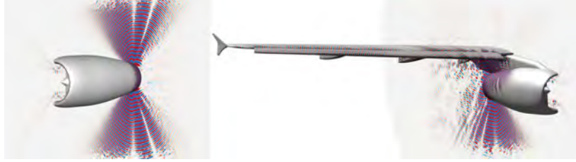
Figure 32: Sound pressure of the isolated (left) and installed (right) engine cases
