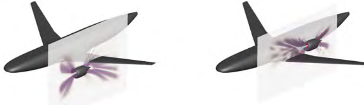
Figure 1: Instantaneous pressure fluctuations with one-sided engine aircraft in the vertical nacelle mid-section plane: UWN configuration (left); OWN configuration (right).
