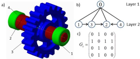
**Fig. 1.** (a)-a gearbox system (b)- its directed graph, and (c)-the corresponding connection matrix.
