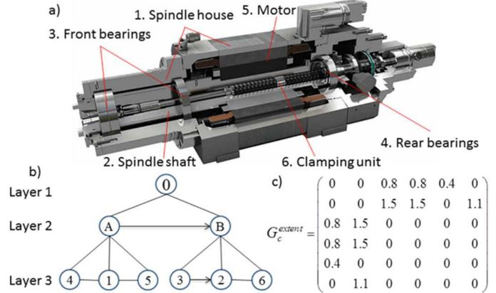
Fig. 4. a- A sketch of an internal motor spindle, b-its directed graph and c-its extent connection matrix.
