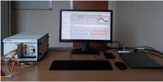
Fig. 6. Waveform platform setup.
