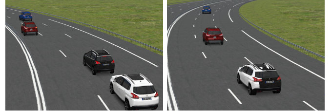
Fig. 5: Verdict visualization with SCANeR studio (left: before cut-in (at 3s), right: after cut-in (at 34s)): Ego (black vehicle), Reference at TIV = 2s (white vehicle), Initial lead vehicle (blue vehicle) and Cut-in vehicle (red vehicle).
