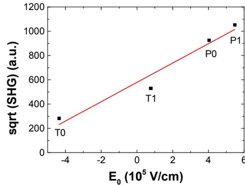
Figure 3. Square root of the initial SHG values from Figure 2 represented versus the static electric field calculated with the fixed oxide charges of each sample from Table I.
