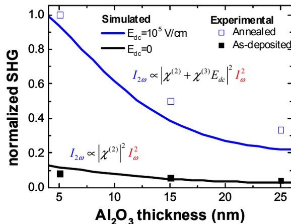
Figure 4. Experimental and simulated SHG intensity versus  $Al_2O_3$  thickness. The measurements were performed at  $45^\circ$  angle for P-input/P-output polarizations. The normalization was done by dividing each set of values (experimental and simulated) with its corresponding maximum value.
