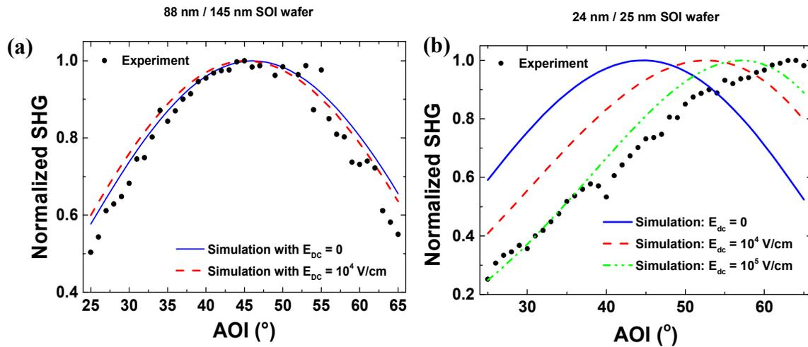
Figure 6. (a) Normalized SHG versus angle of incidence in SOI with 88 nm Si film thickness and 145 nm BOX thickness: model (lines) and experiment (data points). A simulation with a field of  $10^4$  V/cm was added. (b) Normalized SHG versus angle of incidence in SOI with 24 nm Si film thickness and 25 nm BOX thickness: model (lines) and experiment (data points). For the modeling, three different values of  $E_{DC}$  were tested: 0,  $10^4$  V/cm and  $10^5$  V/cm.
