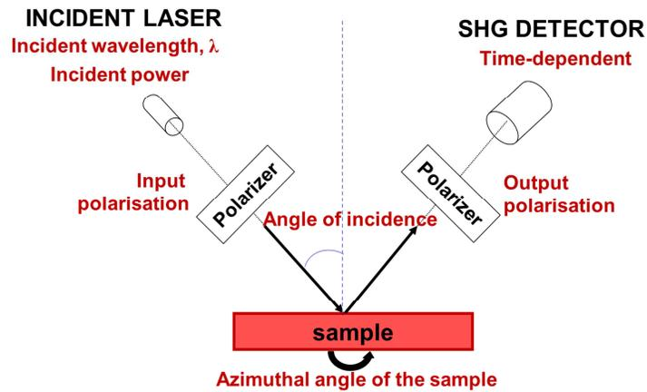
Figure 1. Schematic of the experimental SHG configuration, with the key parameters.
