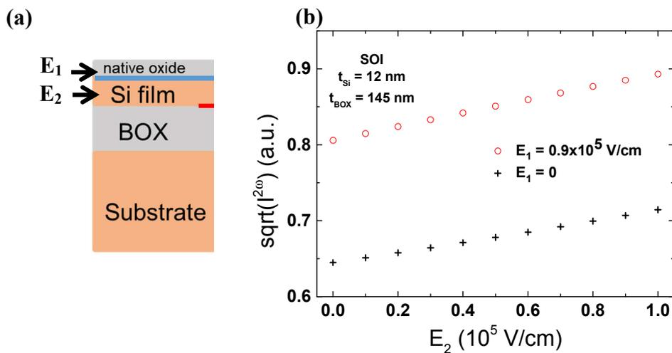
Figure 7. (a) Simulated SOI structure showing the interface between the Si film and the BOX, where the electric fields  $E_1/E_2$  were added at the interfaces with the film. (b) Square root of the SHG versus the electric field at the film-BOX interface.
