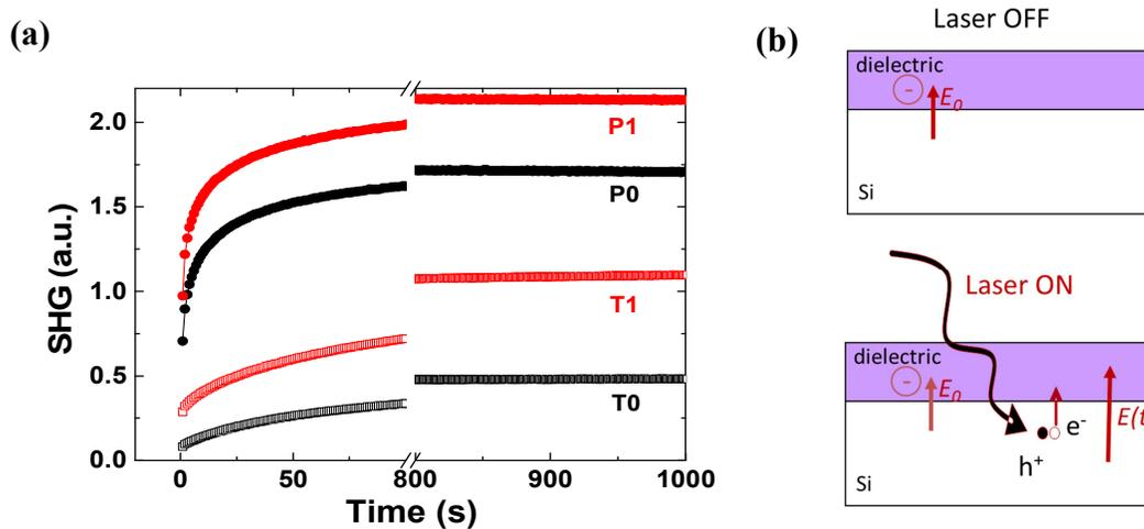
Figure 2. (a) SHG signal versus time measured for four alumina samples with the  $Q_{ox}$ ,  $D_{it}$  values given in Table I. The time scale is broken in order to show both the zoom at the beginning of the measurement and the saturation response. The measurements were performed at  $45^\circ$  incidence angle, for P-input/P-output polarizations. (b) Interface electric field in the sample is modified by the charges generated and injected during the SHG measurement.
