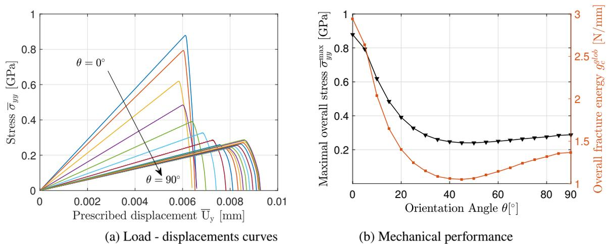
**FIGURE 14** Comparison of the mechanical responses for different orientation angles: the material anisotropic effects are clearly captured. The material orientation strongly alters the mechanical performance as demonstrated by the pic stress and the global fracture energy
