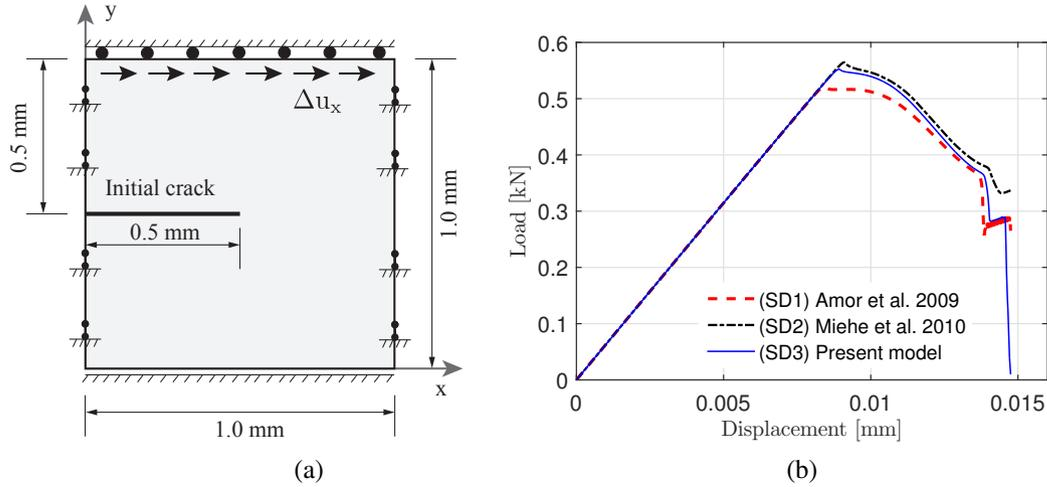
**FIGURE 2** Single edge notched pure shear test sample: (a) geometry and boundary conditions; (b) comparison of load - displacement curves for the different strain split operators. The prediction of the (SD1) model (Amor et al.<sup>5</sup>) is significantly different with respect to the (SD2) and (SD3) models.
