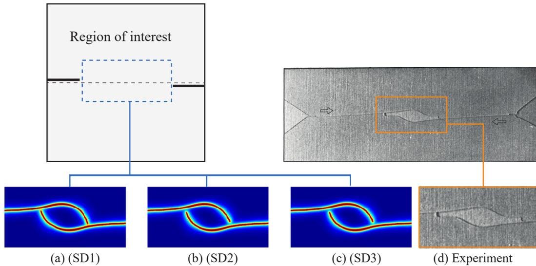
**FIGURE 6** Crack coalescence behavior in the traction test of a doubled notched sample. All three models successfully reproduce the phenomenon of cracks avoiding each other observed in the experiment<sup>47</sup>.
