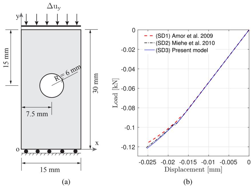
**FIGURE 7** Compression test of a sample containing an hole: (a) geometry and boundary conditions; (b) comparison of load - displacement curves for the different models. The (SD1) model again predicts a lower fracture resistance as compared to the (SD2) and (SD3) models.
