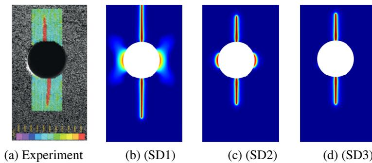
**FIGURE 9** Compressive test: comparison of crack paths predicted by the different strain decomposition schemes with the one of experiment<sup>48,35</sup> for the same loading.
