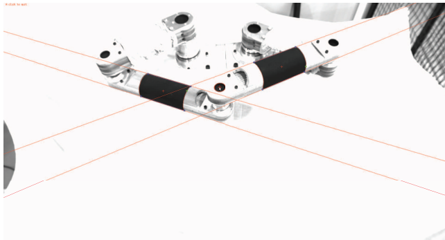
Fig. 11. Tracker for detecting leg edges and end-effector location.
