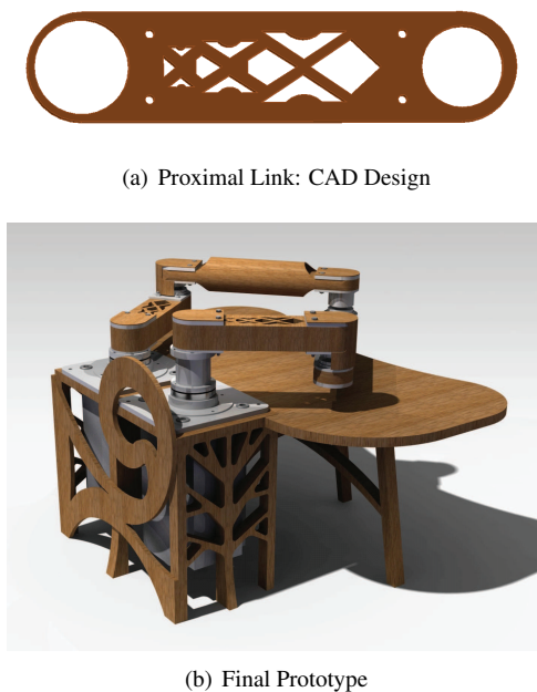
Fig. 8. CAD Design of a wooden five-bar mechanism.
