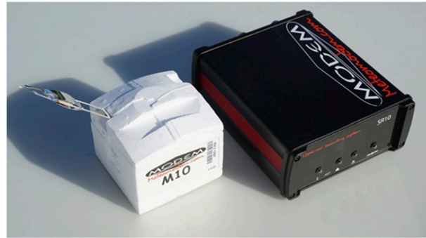
FIG. 1. The Meteomodem M10 radiosonde and its receiver SR10.
