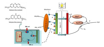
Fig. 4. Schematic of yeast fuel cell system
