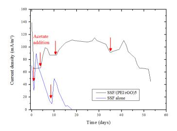
**Fig. 2.** Debit of the electrode with a resistance of 1 k $\Omega$  between the working electrode (either SSF/(PEI/rGO)5 or SSF). The addition of acetate is reported through the red arrows (from [87]).
