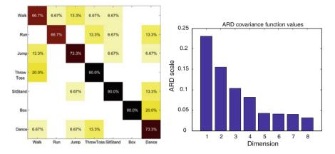
Fig. 3 Left Confusion matrix by using D-SBGPLVM model in combination with SVM on the CMU dataset. Average accuracy: 72.9% Right sorted ARD covariance function values obtained after training the model for the same dataset using the RBF-ARD kernel. Average accuracy: 74.1%
