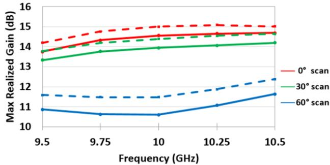
Fig. 10 Evolution of the maximum realized gain versus frequency for different scan angles in the H-plane, without the strips (dotted lines) and with the strips (solid lines)
