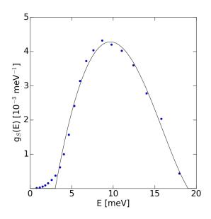
FIG. 4. The Boson Peak of glassy silica at 1673 K, taken from Ref.<sup>17</sup>, reported in non reduced units  $(g(\omega) - g_D(\omega))$ , together with the fit with a 5 degree polynomial
