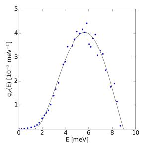
FIG. 1. The Boson Peak of glassy glycerol at 170 K, taken from Ref.<sup>60</sup>, and reported in non-reduced units  $(g(\omega)-g_D(\omega))$ , together with the fit with a 5 degree polynomial
