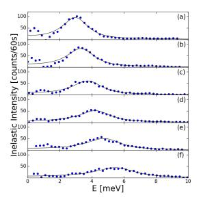
FIG. 2. Inelastic x ray scattering spectra of glassy glycerol as measured at 150 K and reported in Ref.<sup>2</sup> for en exchanged momentum q = 1.3, 1.5, 1.7, 1.9, 2.1 and  $2.5 \text{ nm}^{-1}$  from panel a to f. For the sake of clarity we report only the positive energy exchange side and only the inelastic contribution after subtraction of the elastic line. The black solid lines represent the fit with the string model, where the string distribution has been deduced from the Boson Peak.
