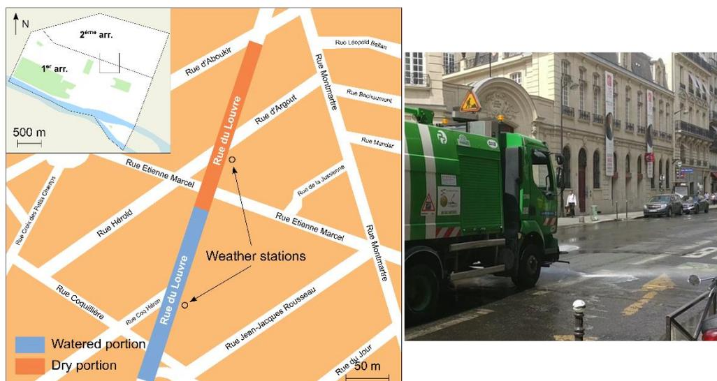
**Figure 3: Illustration of the case and control portions in rue du Louvre (left, adapted from Hendel et al., 2016) and photograph of a cleaning truck performing watering (right).**
