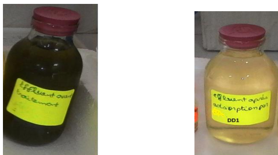
Figure1. Effluent before treatment and after treatment with 13X zeolite synthesised from DD1 kaolin
