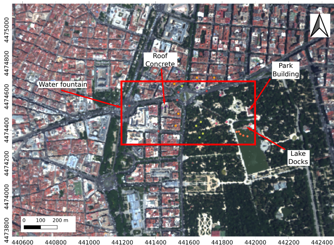
Figure 1. AHS image of Madrid city center from the 4th of July. RGB colours have been composed with AHS reflective bands 7, 4 and 1. The red square delimits the studied area. Colour dots indicate the position of the pixels used to define pure materials in the TRUST methodology, see section 3.
