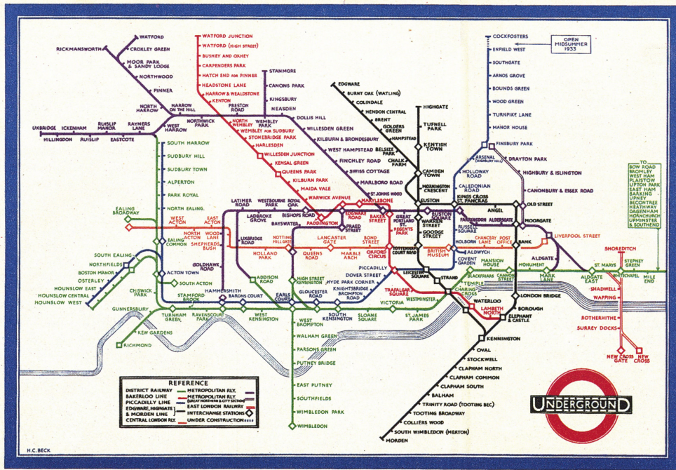
Figure 1. H. C. Beck’s London subway “Tube” map design, as originally published in 1933. This design differed significantly from previous designs in that it introduced a schematized (i.e., heavily generalized) geometry, rather than present the Tube rail lines with planimetric accuracy.
